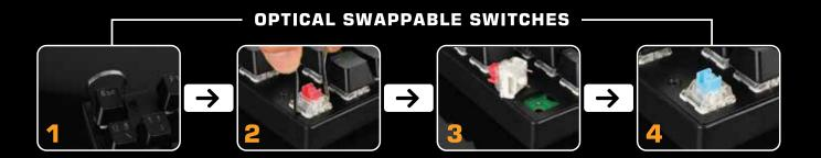
The Trinity keyboard supports Swappable Optical switches. This means that switches are not soldered onto the PCB, and you can easily remove and replace switches.
