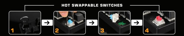
CB-GK-33 Astra keyboard supports Hot Swapping switches. This means that switches are not soldered onto the PCB, and you can easily remove and replace switches with any switches from different brands like Cherry MX, Gateron, Kailh, Outemu.
